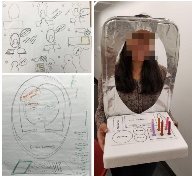
Figure 3: The “Smart Mirror,” created by Mary’s group in 2019 is a system designed to assist people with dementia in putting on make-up by helping them with decision-making through a series of interactive verbal and visual cues.
